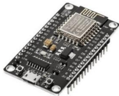
Figure 3. NodeMCU board with integrated ESP8266 Wi-Fi module.
